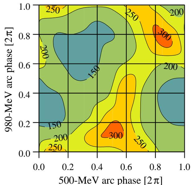
Figure 2: Horizontal beam breakup (BBU) instability threshold current (in mA) determined by the “TDBBU” code, versus betatron phase advance in the 500-MeV and 980-MeV recirculation arcs.
