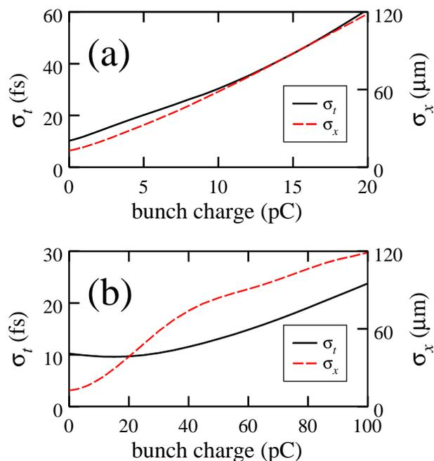
Figure 3: The compressed 980-MeV bunch’s longitudinal and horizontal dimensions versus bunch charge, when coherent synchrotron radiation in the dipole magnets is simulated by the code “elegant”. (a) Maximal compression in both the 500-MeV and the 980-MeV recirculation arcs. (b) Maximal compression in the 980-MeV recirculation arc with isochronous transport at 500 MeV.
