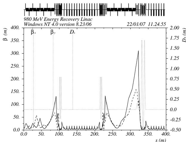
Figure 1: Lattice functions for one half of the 980-MeV energy recovery linac.
