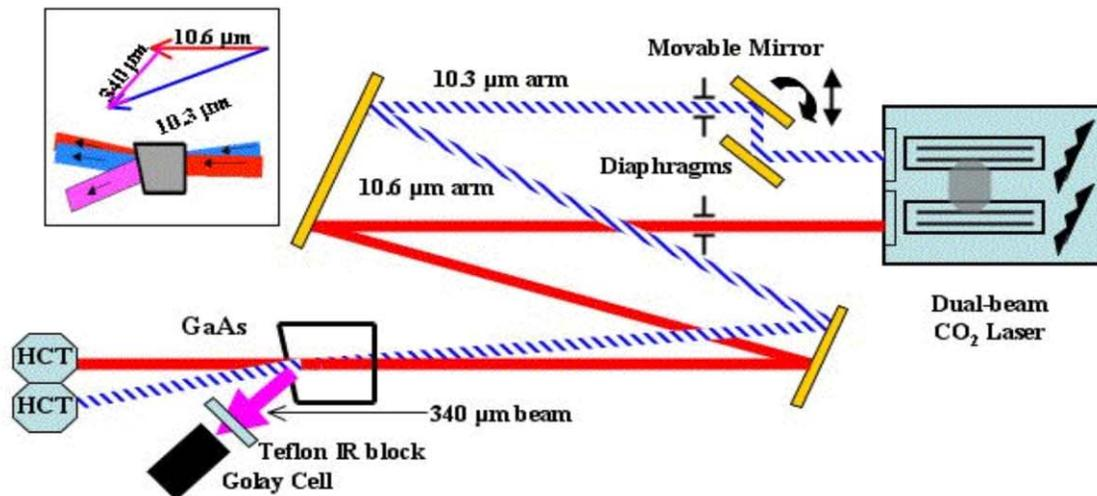
Figure 1: A simplified scheme of a THz DFG source.
