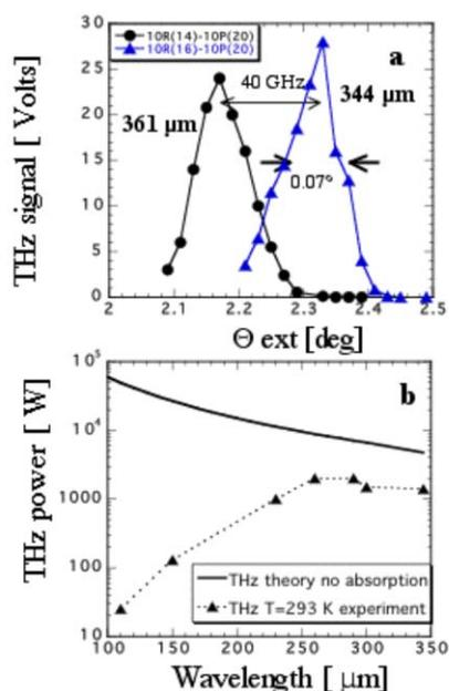
Fig.2 DFG power at 344  $\mu\text{m}$  (triangles) and at 361  $\mu\text{m}$  (circles) versus external phase matching angle  $\Theta_{ext}$  in GaAs (a) and calculated (solid line) and measured (triangles) DFG peak power in the THz range (b).
