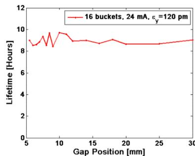
Figure 4: Touschek lifetime as a function of magnetic gap of the in vacuum insertion device. The physical aperture is about 0.3 mm smaller than the magnetic gap.
