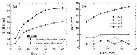
Figure 6: Relation between phase and gap at the maximum merit of flux in the condition (a) circular polarization ( $B_x=B_z$  and out of phase) and linear polarization at  $45^\circ$  ( $B_x=B_z$  and in phase), (b) various harmonic numbers for elliptical polarization ( $B_x \neq B_z$  and out of phase) mode.
