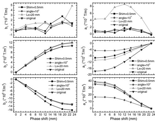
Figure 3: Multipole field variation of the central pole as a function of phase shift under various magnet block arrangements, with  $b_n$  and  $a_n$  as the skew and normal components, respectively.
