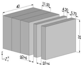
Figure 5: Dimension of optimized magnet blocks and the distance of the end-pole design.
