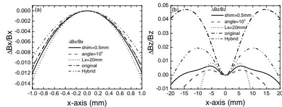
Figure 2: Roll-off of the peak field at (a)  $P=\pi$  ( $B_x$ ) and (b)  $P=0$  ( $B_z$ ) distributed in the horizontal  $x$ -axis, in which phase  $P=2\pi(\Delta z/\lambda_u)$ ,  $\Delta z$  is the phase shift distance in the longitudinal axis and  $\lambda_u$  is the periodic length.
