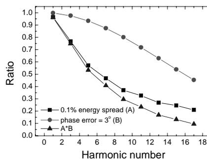
Figure 7: Flux decrease ratio as a function of the harmonic number under a phase error 3 deg, energy spread 0.1%, and the combination factor of phase error 3 deg and energy spread 0.1%.
