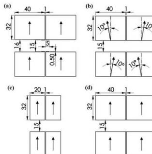
Figure 1: Several methods applied to increase the homogeneity field region: (a) a step shim of thickness 0.5 mm at the block edge, (b) a 10-deg magnetized tilt angle in the V-block, (c) a shortened magnet block dimension in the horizontal axis, and (d) the original block without a step shim.
