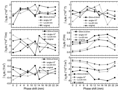
Figure 4: Integral multipole field variation as a function of phase shift for various magnet block arrangements.
