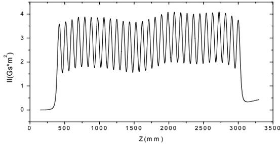
Figure 1: the second integral as function of Z at minimum gap.
