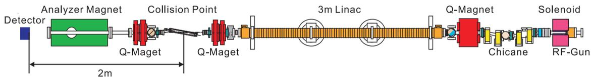
Figure 1: LUCX 40MeV beam line layout
