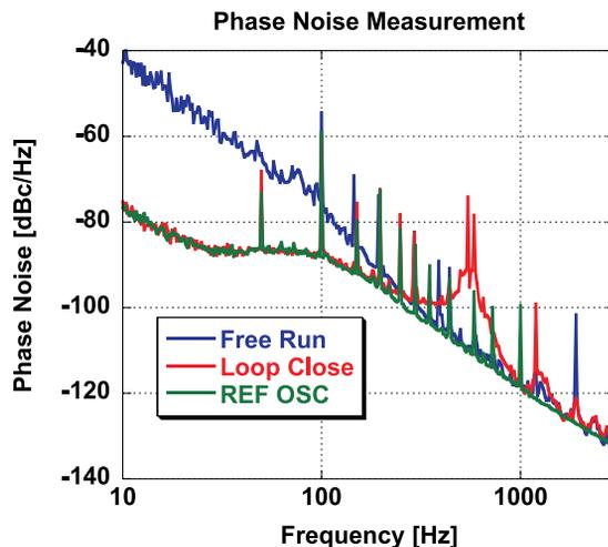
Figure 3: Phase Noise Measurement of Mode-locked Laser
