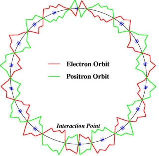
Figure 1: Closed orbits for electrons and positrons.
