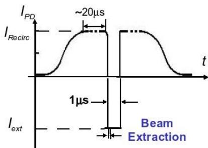
Figure 2: Timing schematic for the pulsed elements for magnetic horizontal extraction.
