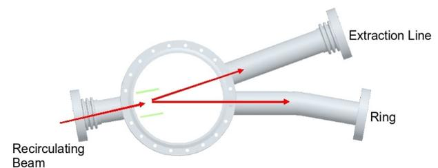
Figure 4: Horizontal extraction using electrostatic bending.
