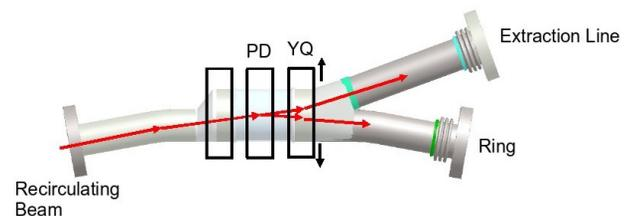
Figure 1: Horizontal extraction using the combined effect of a fast pulsed dipole (PD) and offset quadrupole (YQ) to achieve the net bend angle required.
