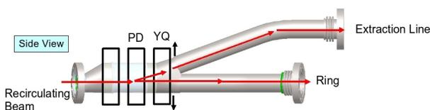
Figure 3: Vertical extraction using the combined effect of a fast pulsed dipole (PD) and offset quadrupole (YQ).
