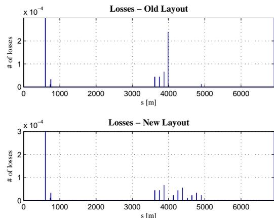
Figure 5: Loss pattern for 400 GeV sweep, old bumper layout (top) compared to the new 2007 layout (bottom).
