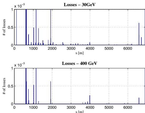
Figure 6: Losses for 30 and 400 GeV; sparks after 11 μs.
