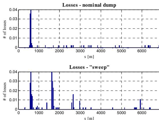
Figure 8: BLM readings during nominal dump and sweep with a 400 GeV fixed target low intensity beam.
