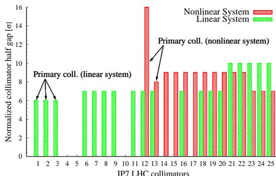
Figure 1: Comparison of the normalized collimator apertures for the nonlinear and the linear collimation systems. In the nonlinear case, the collimators [#1, #11] are not used, and collimators #12 and #13 play the role of primary spoilers at IP7.
