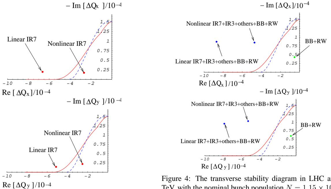
Figure 3: The transverse stability diagram in LHC at 7 TeV, with the nominal bunch population  $N = 1.15 \times 10^{11}$  protons. The points compare the tune shift introduced by the nonlinear and the linear collimation sections IR7.
