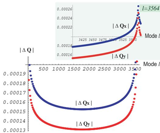
Figure 2: Module of the horizontal ( $|\Delta Q_x|$ ) and the vertical ( $|\Delta Q_y|$ ) coherent coupled-bunch tune shifts as a function of the coupled-bunch mode  $l$  for the case of the nonlinear IR7. The figure on the top shows a zoom of the region  $l \in [3400, 3575]$ . The results have been obtained assuming  $m = 0$  and  $\xi = 0$ .
