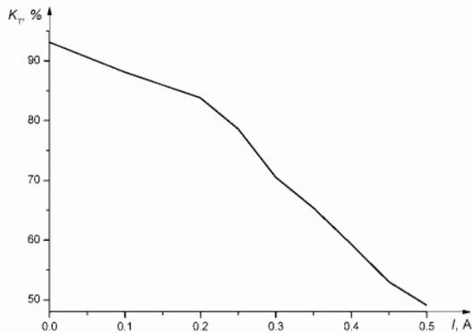
Figure 2: Current transmission coefficient of  $D^-$  ion beam versus input beam current.
