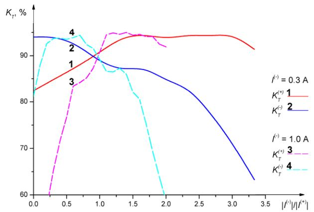
Figure 6: The current transmission coefficient as the function of  $|I^{(-)}| / |I^{(+)}|$ .
