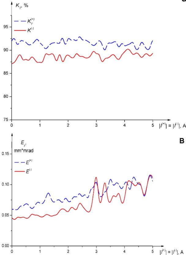
Figure 5: The current transmission coefficient (a) and transverse beam emittance (b) of neutral dual beams versus the input beam current.
