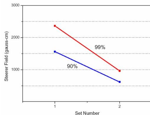
Figure 7: The required magnetic field of the two steering magnet sets: Each case is for 90% and 99% values (The maximum values of the displacement and rotation errors are 50  $\mu\text{m}$  and 17 mrad.).
