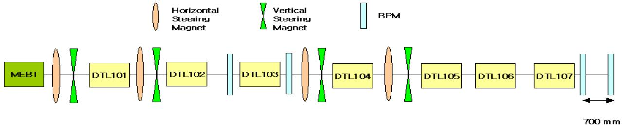
Figure 2: Beam steering in the PEFP linac.
