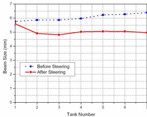
Figure 5: The maximum beam size in the seven tanks after 20 MeV: blue (dotted) line before steering and red (real) line after steering.
