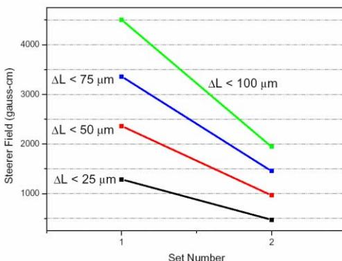
Figure 6: The required magnetic field of the two steering magnet sets: Each case is for different maximum values of the displacement errors (25, 50, 75, and 100  $\mu\text{m}$ ) with a common maximum value of the rotation error of 17 mrad.
