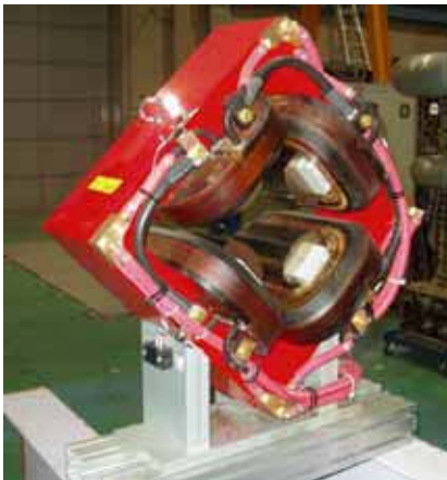
Figure 7: Prototype quadrupole magnet for beam lines
