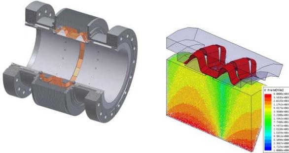
Figure 6: Copper-Beryllium Strip Shielded Bellows.
