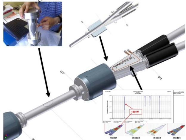
Figure 2: IP1 low- $\beta$  permanent magnet and thin chamber.
