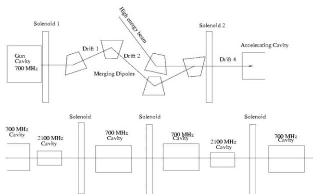
Figure 1: Layout of the injector and linac. The system has two solenoids for emittance compensation, a Z-bend merging system, for 700 MHz accelerating cavities and two 2100 MHz decelerating cavities to minimize the energy spread of the beam.
