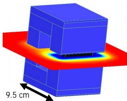
Figure 4. COMSOL 3D simulation of the compact PM dipole to be used in the bench test. The projection of the field strength on the midplane shows the uniformity of the field over the volume of the test cell (2% variation).
