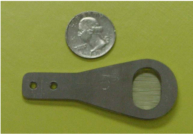
Figure 1: Picture of the wire mesh mask and frame. The tungsten wires are horizontal in the picture. The wires are 500\ \mu\text{m} in diameter with a period of 1270\ \mu\text{m} .
