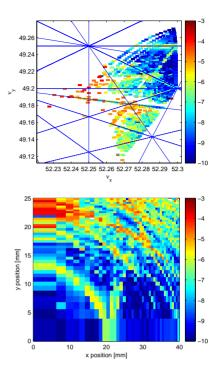
Figure 6: Frequency map for  $Q_x=52.300$  and  $Q_y=49.275$ . Resonances up to fifth order are shown.
