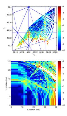
Figure 4: Frequency map for a tune of  $Q_x=52.2810$  and  $Q_y=49.4012$ . Resonances up to fifth order are shown.
