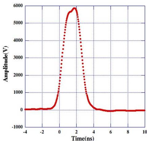
Figure 2: Waveform of the FPG5-3000M output
