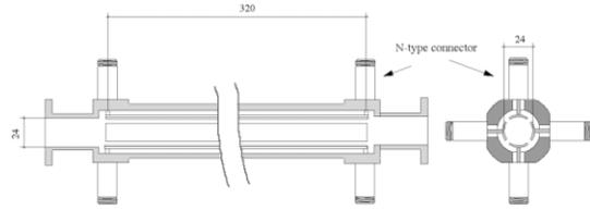
Figure 3: Strip-line electrode used for the beam test
