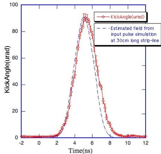
Figure 4: Beam kick profile as a function of the kick pulse timing
