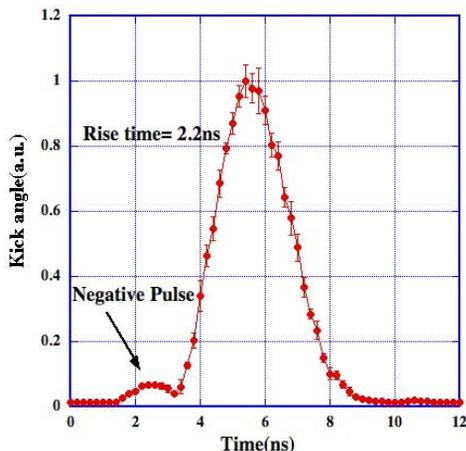
Figure 6: Beam kick profile with waveform compensator
