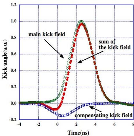
Figure 5: Simulated kick field with waveform compensator
