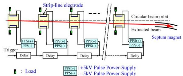
Figure 1: Schematic layout of strip-line kicker system
