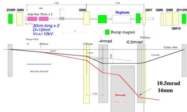
Figure 7: Layout of the beam extraction section for the strip-line kicker
