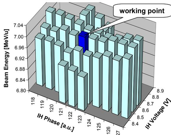
Figure 6: Final beam energy behind the linac as function of the (scaled) IH tank voltage and its rf phase (for  $^{12}\text{C}^{4+}$ ).
