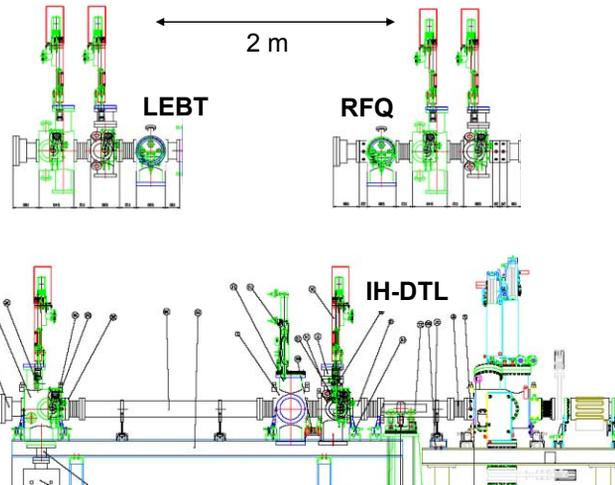
Figure 2: Mobile beam diagnostics benches used during beam commissioning of the different linac sections. The beam enters from the right, respectively.
