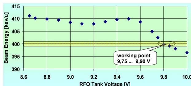
Figure 4: Measured RFQ output energy as function of the (scaled) tank voltage for  $^{12}\text{C}^{4+}$  operation.
