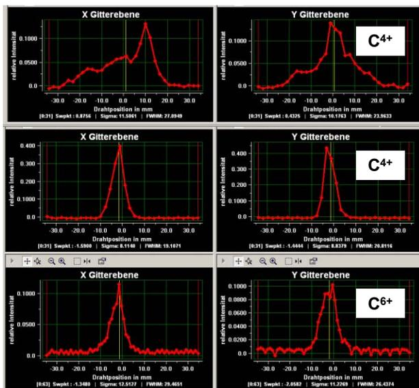
Figure 7: Horizontal (left) and vertical (right) LEBT beam profiles (top), behind the IH-DTL, and before synchrotron injection.
