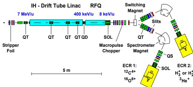
Figure 1: Layout of the HIT injector linac [2]. QS, QD, and QT means quadrupole-singlet, -doublet and -triplet, respectively, SOL means solenoid magnet; focusing and steering magnets (green), profile grids and tantalum screen (red), and beam current monitors (blue).
