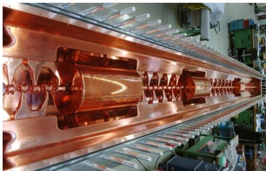
Figure 5: Open IH cavity after copper plating and installation of the drift tubes; the beam enters from the left.
