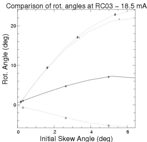
Figure 3: Comparison of skew angles between experiment and simulation as a function of initial skew angle. \*:S-G, #:K-V, o:e-gun, e:experimental.
