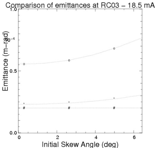
Figure 4: Comparison of emittances as a function of initial skew angle. \*:S-G, #:K-V, o:e-gun.
