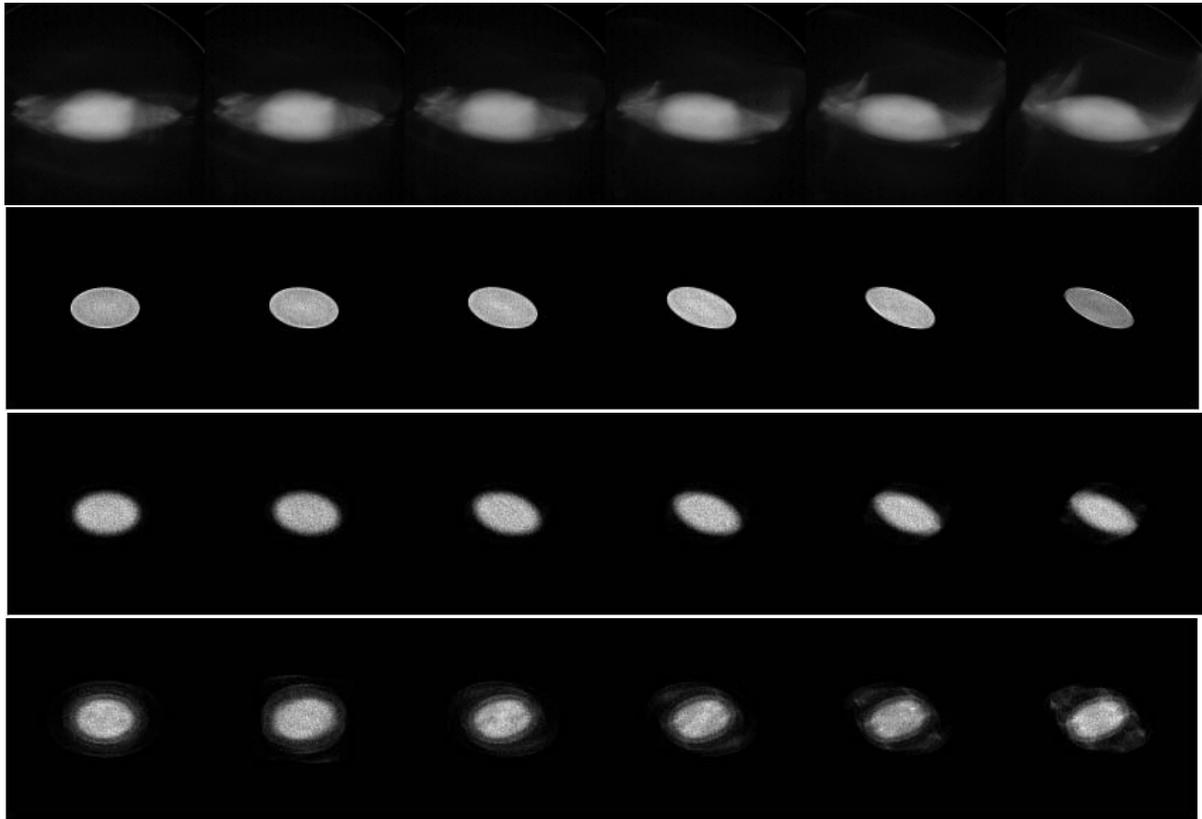
Figure 2: Comparison of experiment (first line) and simulation (K-V, semi-gaussian and e-gun initial distributions respectively.)
