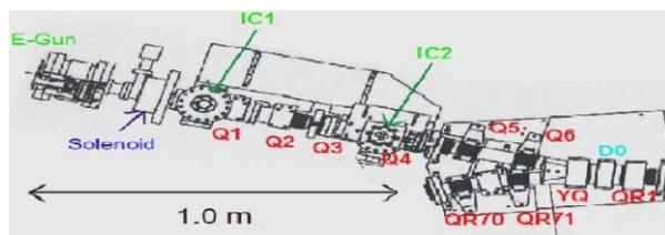
Figure 1: Schematic of the injection section of UMER. The skew quadrupole is located in Q6.
