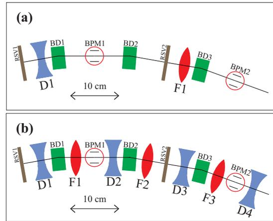
Figure 1: UMER lattices with (a) one quadrupole per ring section ( $S=128$  cm) - one FODO cell shown, and (b) four quadrupoles per ring section ( $S=32$  cm) - almost four complete FODO cells shown. See text for explanation of labels and Table I for beam parameters.
