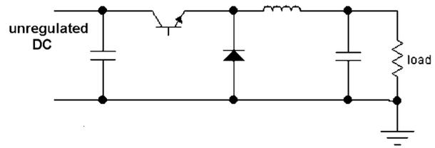
Figure 4. The basic architecture of a switching buck regulator, or DC-DC down-converter, shows the series switch, the freewheeling diode, and the filter inductor.
