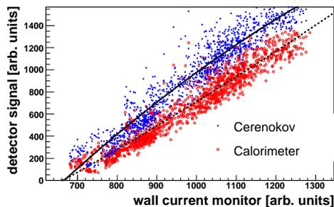
Figure 5: Cerenkov and calorimeter signals plotted as a function of beam charge
