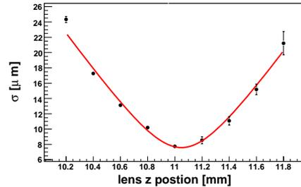
Figure 3: Laser waist scan using the Cerenkov detector.
