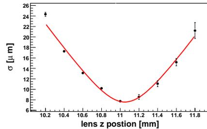
Figure 3: Laser waist scan using the Cerenkov detector.
