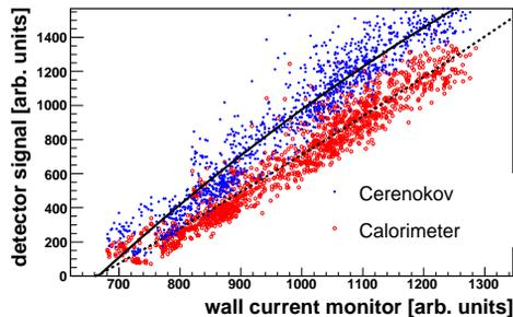
Figure 5: Cerenkov and calorimeter signals plotted as a function of beam charge
