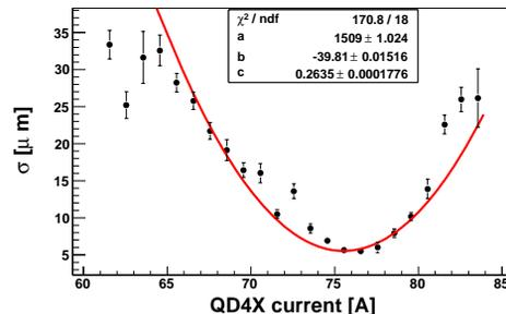
Figure 6: LW measured vertical beam size as a function of quadrupole QD4X current.
