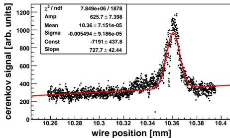
Figure 2: Cerenkov detector signal as a function of laser beam vertical position.
