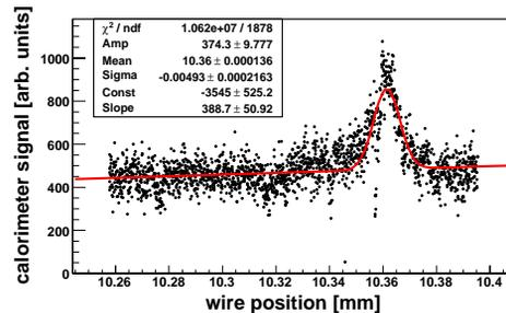
Figure 4: Calorimeter detector signal as a function of laser-beam vertical position.
