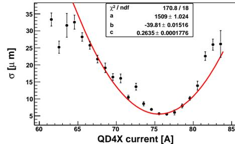
Figure 6: LW measured vertical beam size as a function of quadrupole QD4X current.
