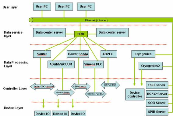
Figure 1: The infrastructure of NSRRC utility control system.
