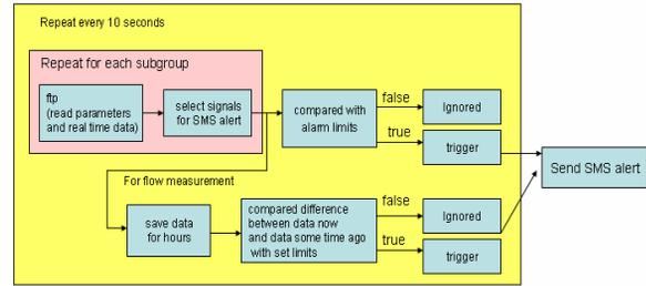
Figure 2: The block diagram of design of SMS alert program.
