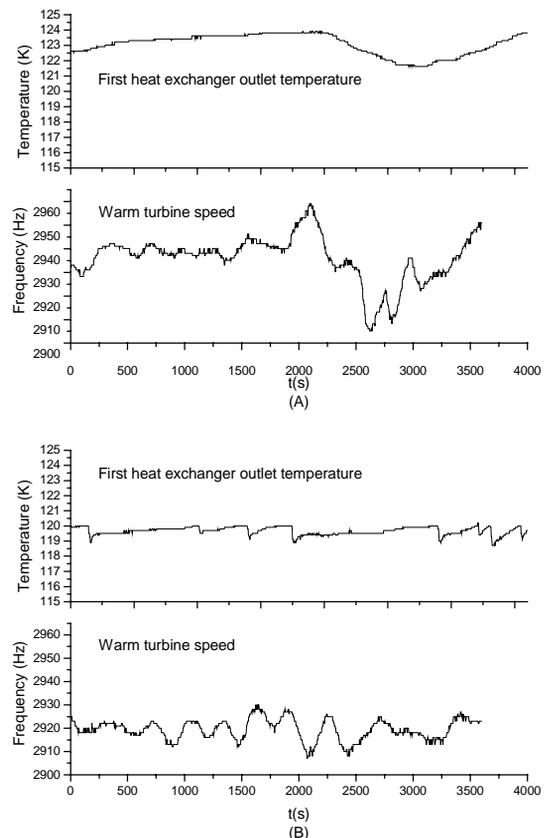
Figure 1: (A) The variations for first heat exchanger outlet temperature without LN<sub>2</sub> pre-cooling, (B) The variations for first heat exchanger outlet temperature with 120K LN<sub>2</sub> pre-cooling
