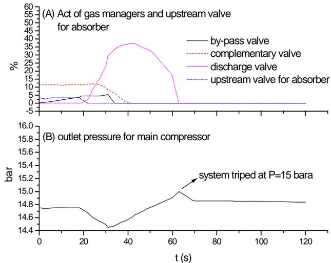
Figure 4 (A) The actions of gas managers and upstream valve for absorber, (B) Variation of outlet pressure for main compressor
