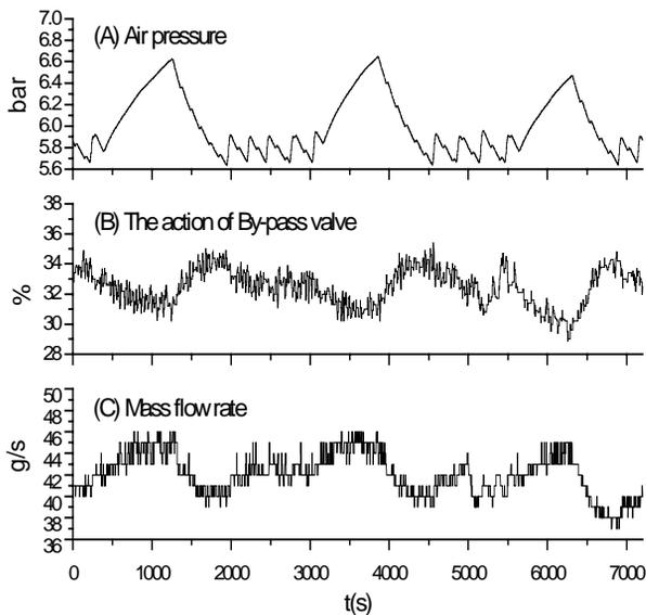
Figure 2: (A) The pressure of control air, (B) The variation of by-pass valve, (C) The variation of mass flow rate.
