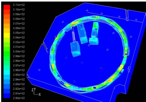
Figure 4: Simulated temperature contour for the booster area.
