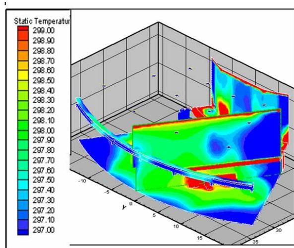
Figure 1: Simulated temperature contour for the experimental hall.
