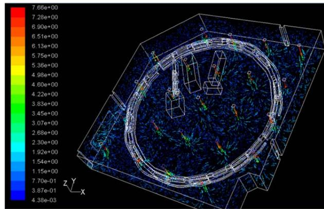
Figure 5: Simulated air velocity vectors for the booster area.
