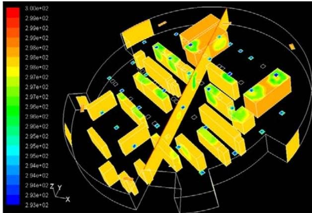
Figure 3: Simulated temperature contour for the technical zone.
