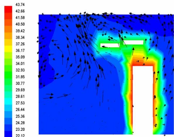
Figure 2: Simulated results of one cross section of the storage ring tunnel.
