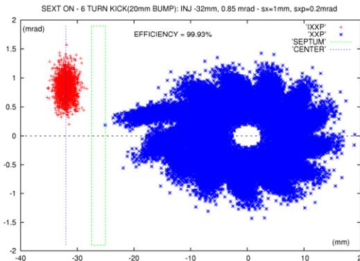
Figure 4: SESAME Injection with  $3 \mu\text{m}$  Ti coating thickness.
