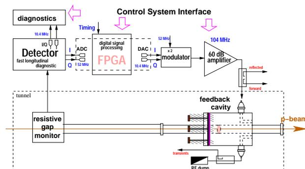
Figure 1: System components of the HERA-p longitudinal coupled bunch feedback system.
