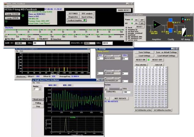
Figure 3: User interface of the longitudinal coupled bunch feedback system at HERA-p.
