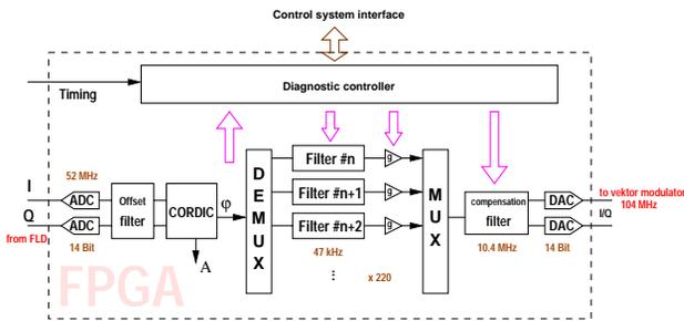
Figure 2: Details of the algorithm implemented in FPGA.
