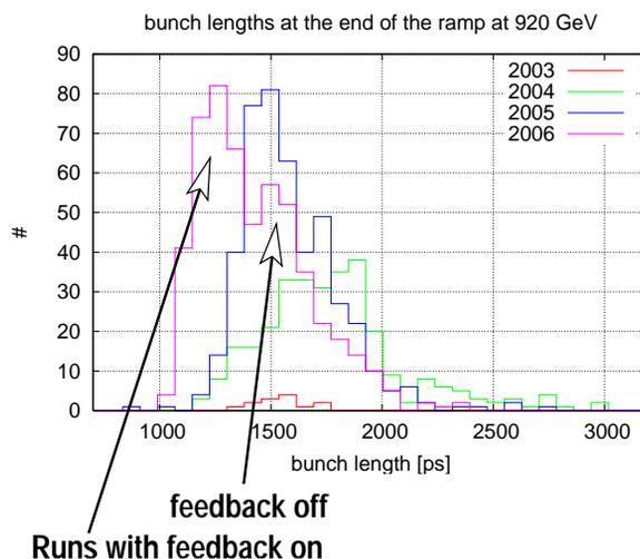
Figure 4: Statistics of bunch lengths for different years of operation of HERA. The bunch length is measured as FWHM of the charge profile of a signal of a resistive gap monitor. In 2006 the feedback system was commissioned and the reduction of bunch length at 920 GeV is visible.
