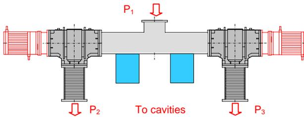
Figure 2: The binary cell consists of a pair circulators with dummy load connected together by shunt tee with integrated phase shifters.
