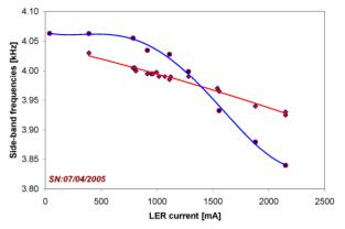
Figure 4: Synchrotron frequency measured from the first (blue) and the second sideband (red) in the beam spectrum.
