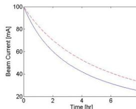
Figure 6: Example beam decay profile with bunch-lengthening (red dash) and without (solid blue).
