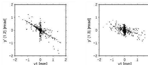
Figure 1: Vertical beam-centroid coordinates at first BPM of 100-MeV H<sup>+</sup> line, computed from data of first two BPMs (left) and from data of first and last BPM (right).
