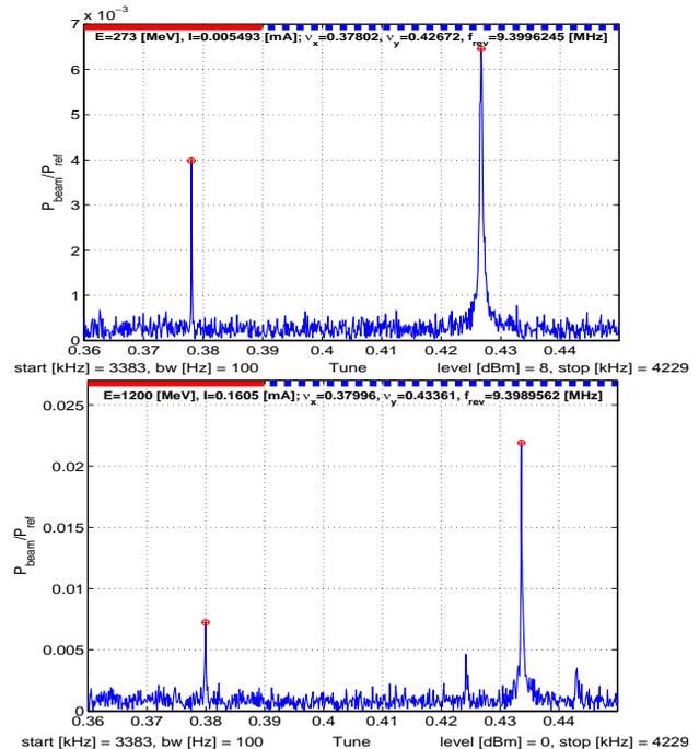
Figure 3: The measured betatron tune signals. The upper plot shows the measured tunes at the injection energy of 273 MeV with about  $5 \mu\text{A}$  of stored beam current; the lower plot shows the measured tunes at the highest extraction energy of 1.2 GeV with about  $150 \mu\text{A}$  of stored beam current.
