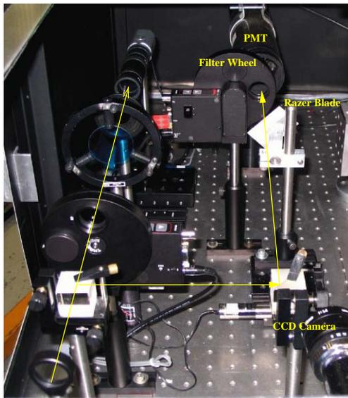
Figure 2: The optical detection system. The optical beam from a dipole synchrotron port passes a space filter (a razor blade) before being detected by a photomultiplier tube.
