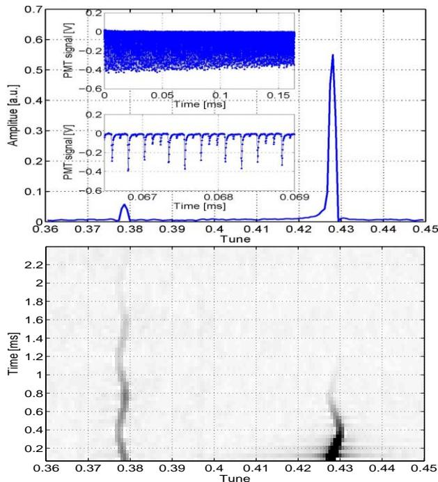
Figure 4: The betatron tunes measured using a real-time oscilloscope. In the upper plot, both tunes,  $\nu_x = 0.378$ ,  $\nu_y = 0.428$ , are plotted together with the corresponding time-domain signals: the upper inset shows a full slice of time domain signal used for FFT analysis; the lower inset shows a selected portion with visible peak modulation. The lower plot shows the evolution of betatron tunes after excitation.
