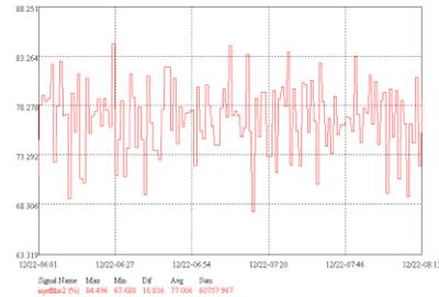
Figure 4: Injection efficiency during top-up mode operation.
