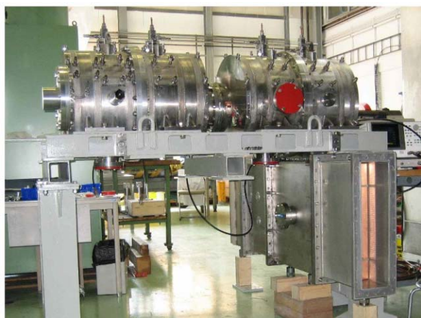
Figure 4: CCDTL prototype from BINP Novosibirsk and VNIITF Snezhinsk.
