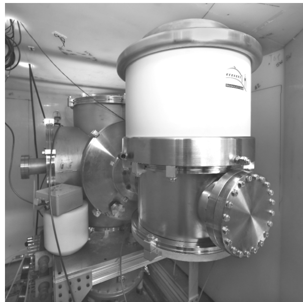
Figure 3: The 10^{11} n/s D-D co-axial neutron generator mounted in one of the P&IST group neutron test stands. The neutron generator is 80 cm tall with the pumping chamber and 40 cm in diameter.
