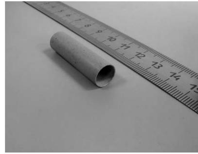
Figure 3. Ceramic waveguide layer made of BST-MgO (BSM) ferroelectric with wall thickness 600  $\mu$ m, diameter 10 mm and length of 4.5 cm. The sample was fabricated for the 11.424 GHz tunable DLA structure project.
