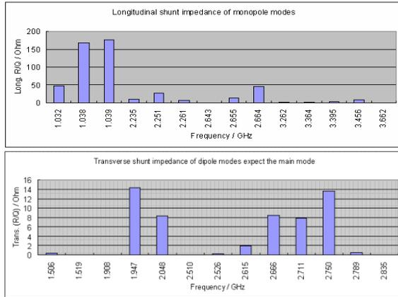
Figure 5: Shunt impedance of LOM's and HOM's
