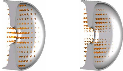
Figure 1: Magnetic (left) and electric (right) field distribution of the deflecting mode in a cavity. Transverse electric fields are introduced due to the beam iris. The deflecting mode is a hybrid mode between TM and TE.
