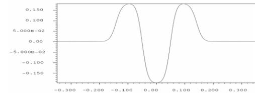
Figure 4 : Longitudinal electric field distribution of  $TM_{110}$ -like  $\pi$  mode, at  $r = 10$ -mm along  $z$ .
