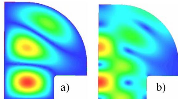
Figure 1: Geometry of our test cavity and false-color plots of the a) E and b) H field patterns for the  $TE_{013}$ -like mode. The left edge is the symmetry axis, and the bottom edge is the face of the test sample.
