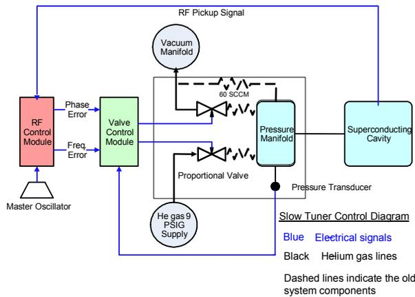
Figure 2: Slow tuner system detailed diagram. Flow restrictors and bypass leak shown in dashed lines.
