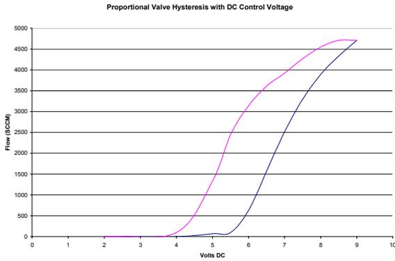
Figure 3: Valve control curve in DC mode.
