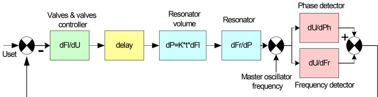
Figure 5. Slow tuner system control block diagram
