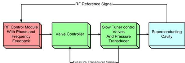
Figure 1: Block Diagram of the slow tuner system.
