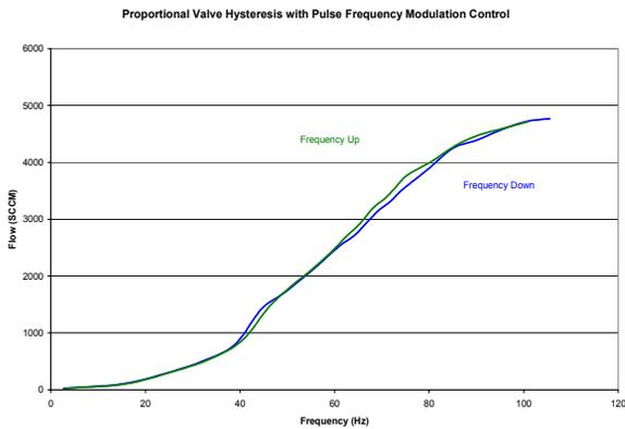
Figure 4: Valve control curve in PFM mode.
