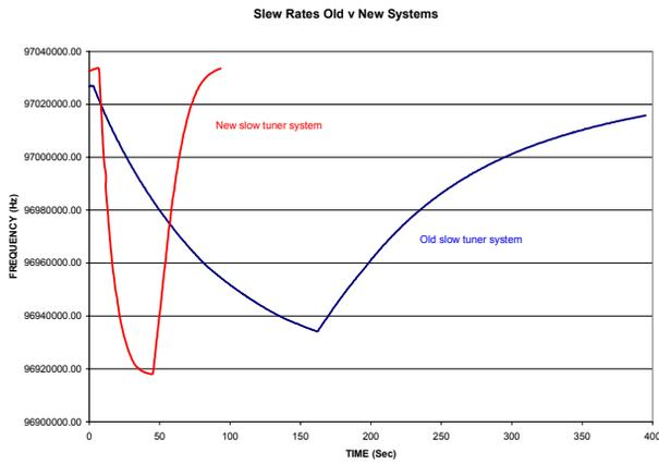
Figure 7: Improvement in the frequency slew rates between the old system and the new prototype system.
