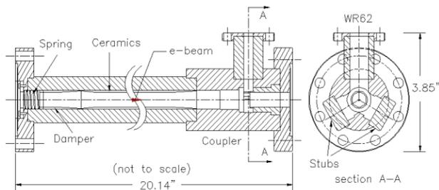
Figure 8: Assembly drawing of the 15.6GHz power extractor with a 2-stub coupler design.
