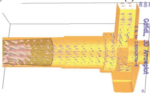
Figure 6: Half model of part of extractor with taper and 2-stub coupler. The fields are induced by a single  $\delta_z=3\text{mm}$  bunch in a short (3cm) regular dielectric.
