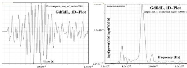
Figure 7: Signal and its spectrum induced in the output port of the 2-stub coupler by the 3mm, 100nC bunch passed through 3cm regular dielectric, tapering and coupler.
