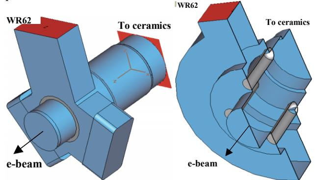
Figure 3: Two-stub (on the left) and four-rod (on the right, one half) couplers designed with the MWS code.
