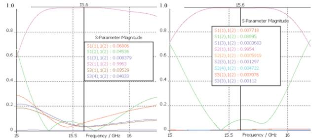
Figure 4: S-parameters for the two-stub coupler (on the left) and four-rod coupler (on the right). Transmission coefficient is  $S_{21} \equiv S_{21}(1)1(2)$ .
