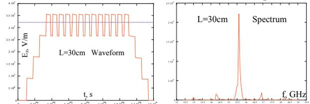
Figure 1: RF envelope of the longitudinal field and its spectrum.  $\delta_z=3mm$ ,  $q=40nC$ ,  $N_b=16$  bunches. The horizontal dashed line corresponds to the formula (1).
