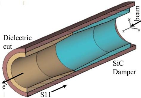
Figure 2: SiC damper (on the right end) for reflected parasitic waves as seen from the regular ceramic tube.  $S_{11} = -27\text{dB}$  at resonant dipole mode frequency 14.2GHz.
