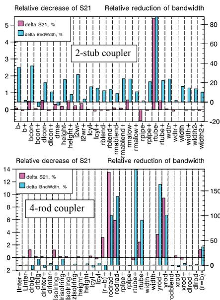
Figure 5: Relative reduction [%] of the transmission (left ordinate) and bandwidth (right) for the two coupler designs vs one-by-one dimensional variations ( $\pm 25.4\mu\text{m}$ ).
