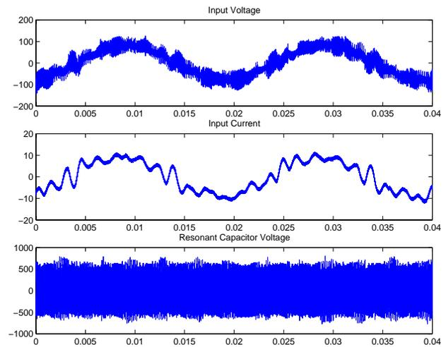
Figure 4: Initial Experimental Results showing an arbitrary phase voltage and current and the resonant capacitor voltage
