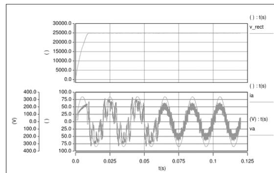
Figure 2: Input Current Waveform With State Biasing Enabled After 60ms)
