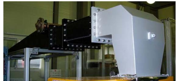
Figure 12: Waveguide and 1 MW CW RF dummy load.
