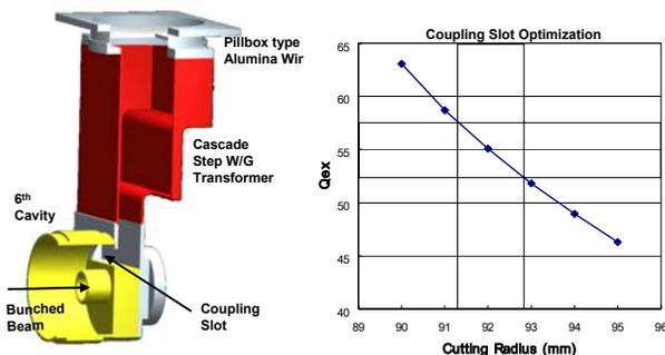
Figure 6: Schematics of the RF output circuit and dependencies of Q<sub>ex</sub> on the size of the coupling slot.
