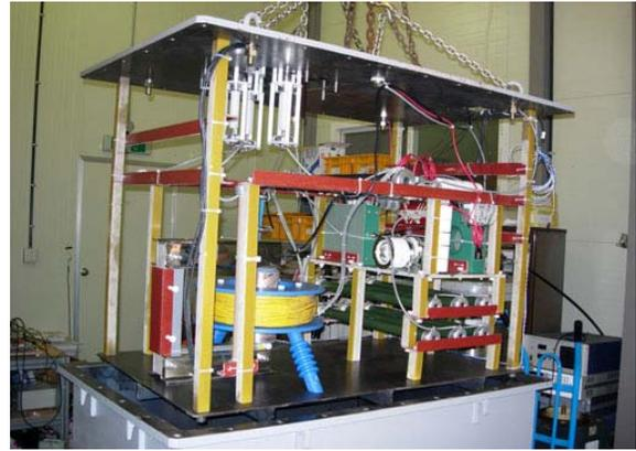
Figure 11: Cathode heating and pulse power system.
