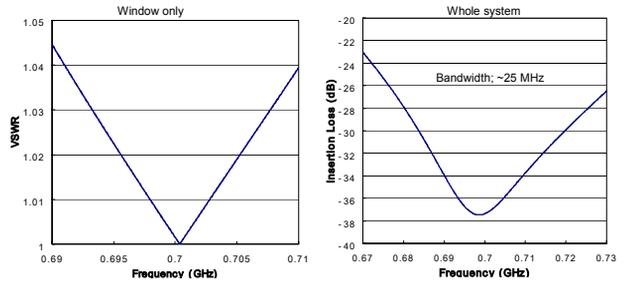
Figure 7: RF characteristics of the RF output circuit.
