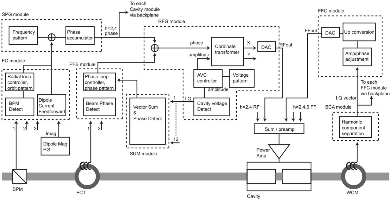
Figure 1: Block diagram of RCS LLRF system
