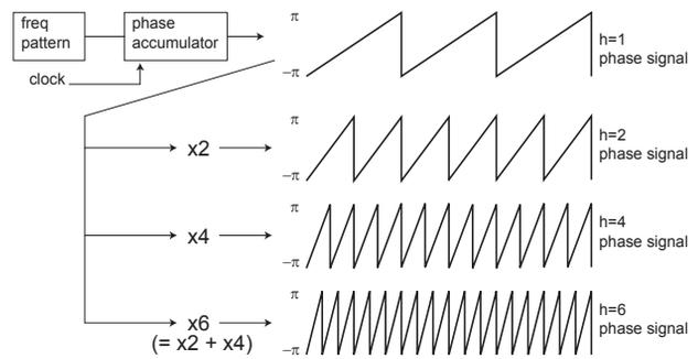
Figure 2: Direct Digital Synthesis (DDS)
