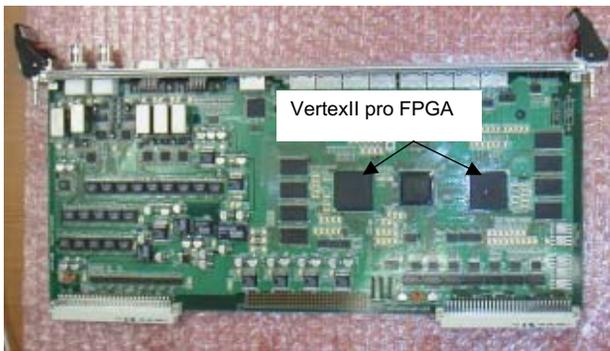
Figure 3: RFG (RF generation) board
