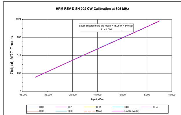
Figure 2: RF Channels 0-6, after calibration
