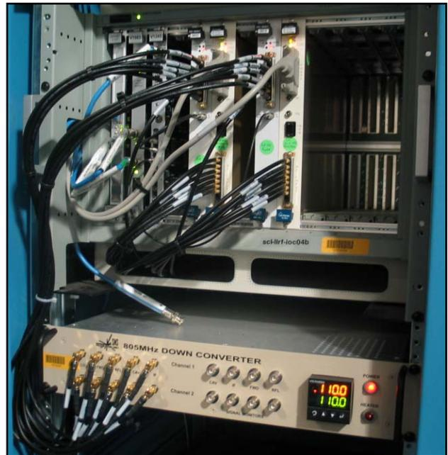
Figure 3: Each rack in the Superconducting Linac contains LLRF control hardware for two RF systems. The VXI crate contains (from left) an IOC running the VxWorks OS, a utility module, a timing module and two HPM/FCM pairs.
