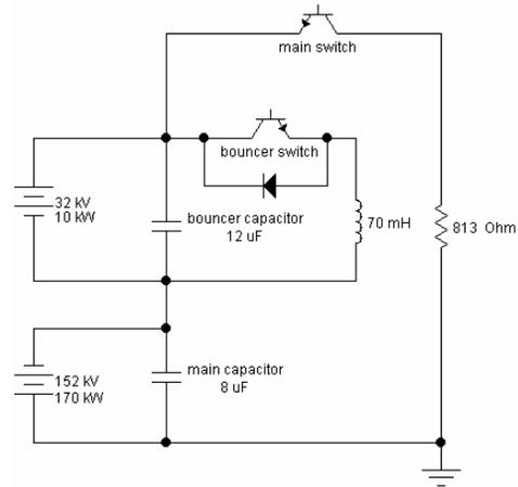
Figure 4. Hard-switch circuit, including bouncer to give flat pulse.
