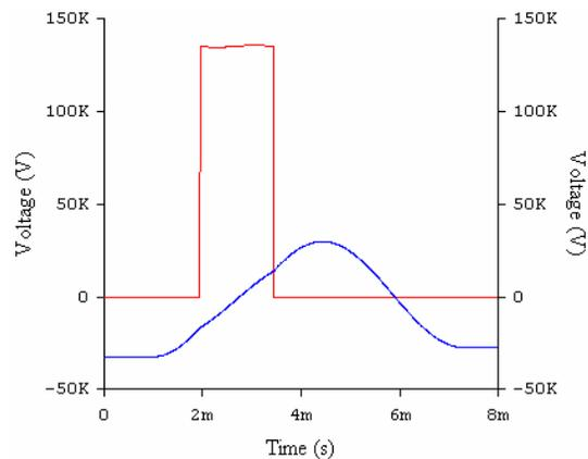
Figure 5. Voltages in bouncer circuit. Upper trace, output voltage; lower trace, voltage across bouncer capacitor.
