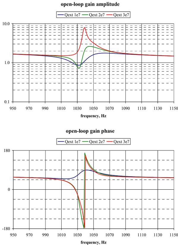
Figure 4: Open-loop Bode plot for different values of passive cavity quality factor (50 mA beam current).
