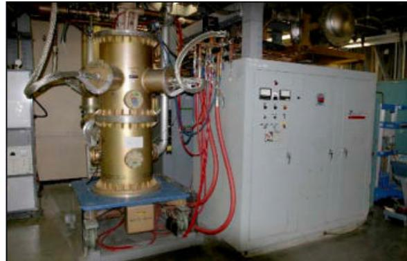
Figure 1: 201 MHz cavity amplifier and filament supply for the Burle 7835 triode.
